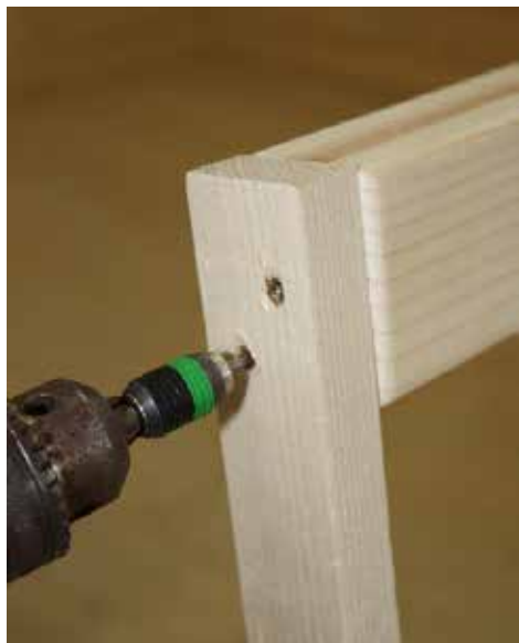
Remove transport strip from the door frame
