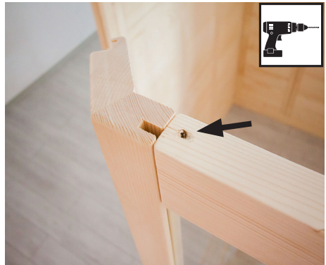
3 mm drill bit, 1 screw 4 x 70 mm
