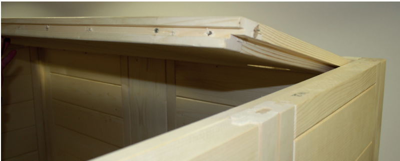
Fig. 17: Installing the roof element in the front
